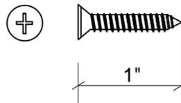
Used to mount 8" Aluminum Wrap Around hinges.
