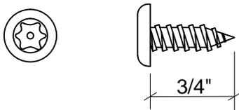
Used for bracket, shoe and headrail connections to plastic components.
