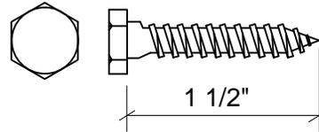
Used for leveling pilasters on uneven flooring.
