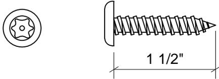
Used for bracket, shoe, and headrail connections into wall or floor.
