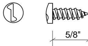
Used to mount hook and bumper/door bumper to doors.
