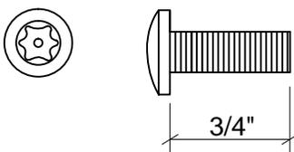
Used to join hardware to plastic components.
