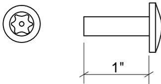
Used to join hardware to plastic components.
