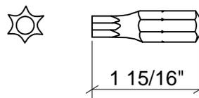
Drill bit for torx and thru-bolts.
