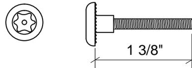
Used to mount door pull to slide latch.
