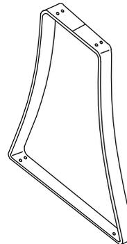
Pedestal fabricated of 2" wide, 16 ga. brushed stainless steel formed into the shape of a trapezoid. 14" long bottom with (2) mounting holes. 16-1/4" high. (4) holes for fastening on top flange.
